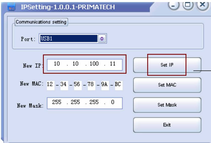
Step 3. Restart the printer, the new ip should work, user can check it on the self test page.
